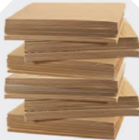
Corrugate Also called fiberboard; made from a fluted sheet of paper and one or two liners of corrugate.
